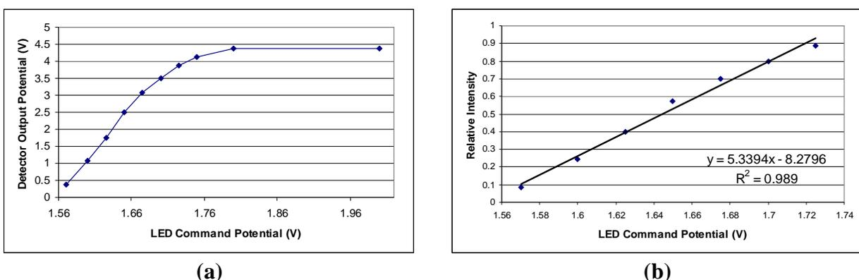
**Figure 3(a)** Calibration response of red LED/photoreistor pair.
