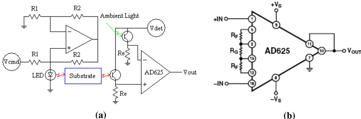
**Figure 2(a)** modification of circuit shown in Figure 1 consisting of an alternative detector circuit which uses an instrumentation amplifier to cancel ambient light.
