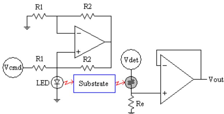
**Figure 1** Schematic of voltage controlled current source (left) which powers the emitter (LED) and a simple detector circuit composed of a detector device (photoresistor in above schematic) and a voltage follower amplifier.
